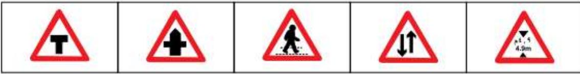
T-intersection ahead (you will need to stop) | Intersection ahead (slow down and prepare to stop) | Pedestrian crossing ahead | Two-way traffic | Maximum headroom at hazard ahead
