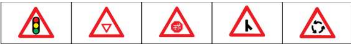
Traffic signals ahead | Give Way sign ahead | Stop sign ahead | junction ahead (you will merge with other traffic) | Roundabout ahead
